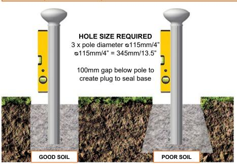
A <u>much larger foundation may be required</u> if soil is poor/sandy to prevent bollards being pushed over or removed/stolen. Try and taper out towards the bottom so the base section of concrete is larger than the top section as per this image
