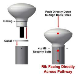
USING 2 PIN SECURITY DRIVER BIT
