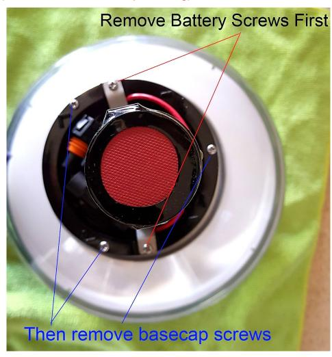
**STEP 3** - Slowly pull out the base cap from the base section without pulling on the solar panel cable to hard.
