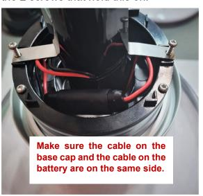
**STEP 10 -** Tuck the cables underneath the metal brackets and place the plug inside the base cap.
