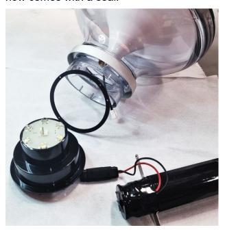
**STEP 6 -** Reconnect the solar panel cable making sure the connector is locked on firmly.
