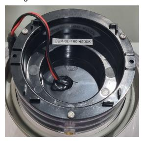
**STEP 9 -** Add new battery with feet sitting within the moulded feet stays and re-insert the 2 screws that hold this on.
