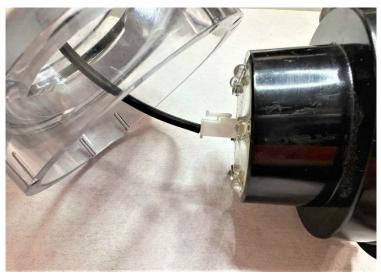
STEP 4 - Disconnect the solar panel cable from the base cap.
